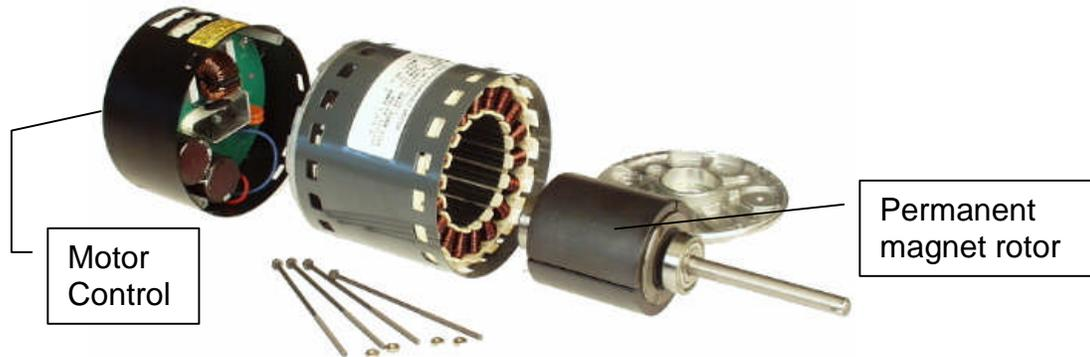
The motor is essentially a three phase motor with a permanent magnet rotor. The permanent magnet rotor contributes to the electrical efficiency of the ECM and also to its sensor-less ability to control the rpm (revolutions per minute) and commutation (when to alternate the cycle). Typical DC motors require brushes to provide the commutation function. This is where the motor gets the name brushless DC motor.
