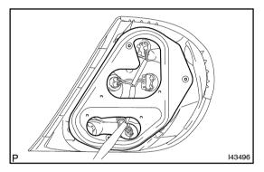
(c) Remove the rear combination lamp gasket RH.
