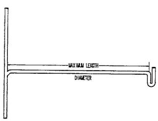
NOTE: THESE DIMENSIONS ARE FROM THE VENT TO THE WEIR OF THE TRAP ALONG THE DEVELOPED LENGTH AND NOT GREATER THAN ¼ INCH PER FOOT.
