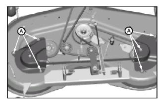
Remove six cap screws (A) and left and right belt shields.
