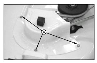
3. Remove three cap screws (A) and belt shield.
