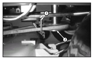
10.Put mower drive belt on engine drive sheave (J). Make sure belt is routed through both belt guide loops (I).
