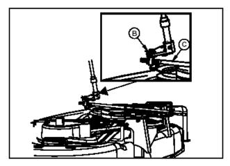
Remove spring locking pin and washer (B) to remove adjustment link and engagement rod (C) from arm.
