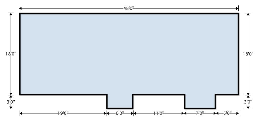
This is the concrete pad layout. It will be two (2) feet wider then the overall building for a total of 18' x 48'
