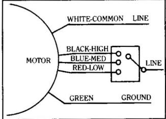
Standard wiring color codes as used by FASCO and most other manufacturers for Shaded-Pole motors.
