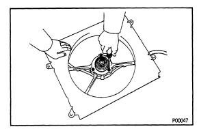
2. REMOVE FAN MOTOR Remove the screws and fan motor.
