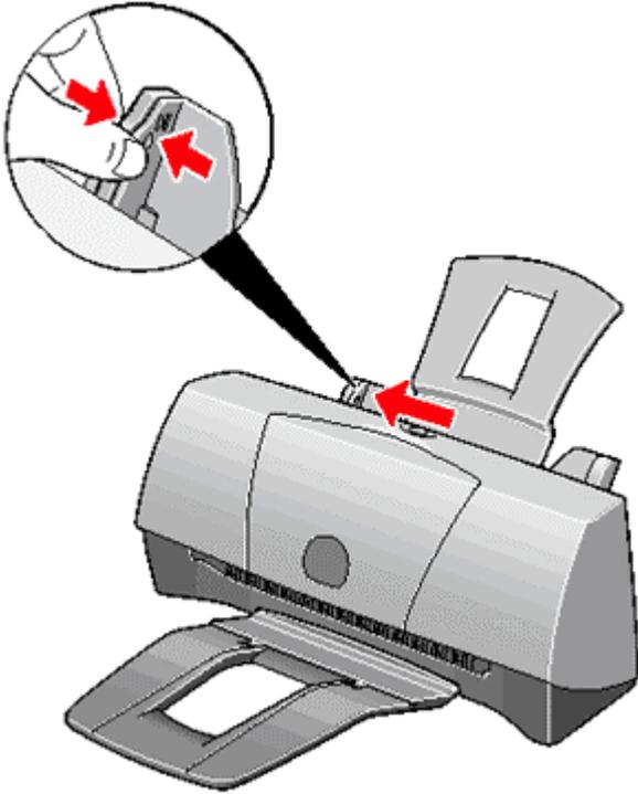
2. Insert the stack of paper with the print side up and adjust the paper guide.
