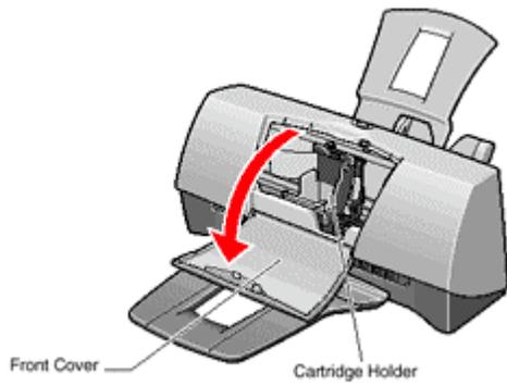
2. Make sure the blue lock lever on the cartridge holder is raised.
