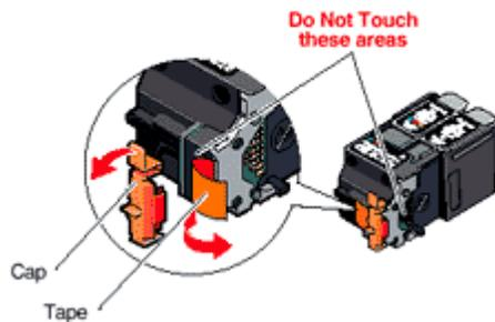
5. Set the cartridge into the cartridge holder.
