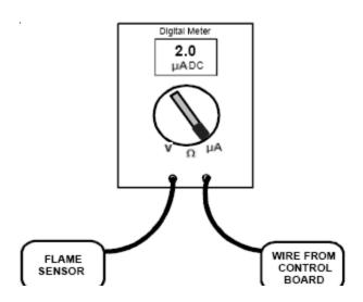
Place the unit into a heating cycle.
