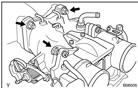
(I) Remove the 3 nuts, throttle body and gasket.
