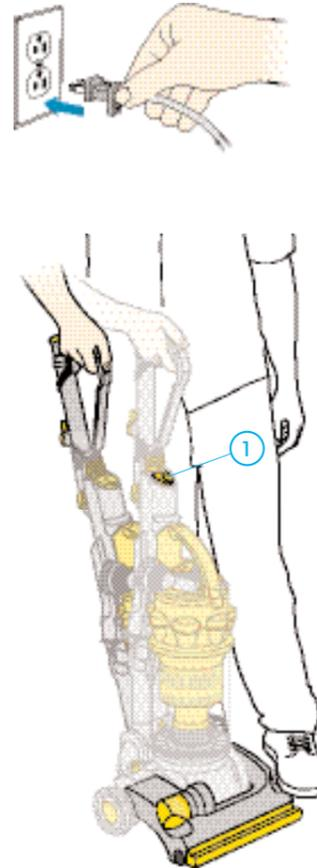
After plugging machine into mains, press on/off button **1**, push cleaner head down with foot and pull handle towards you.
