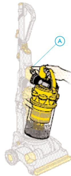
The filter may require washing more frequently than 6 months based on individual vacuuming habits. Press cyclone release button **A** to release cyclone pack.
