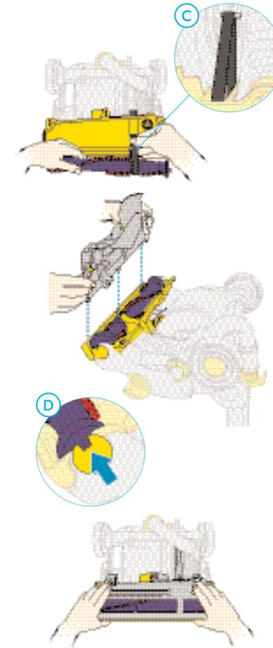
**C** To replace the belt, remove the brushbar, loop belt around brushbar and feed through hole.
