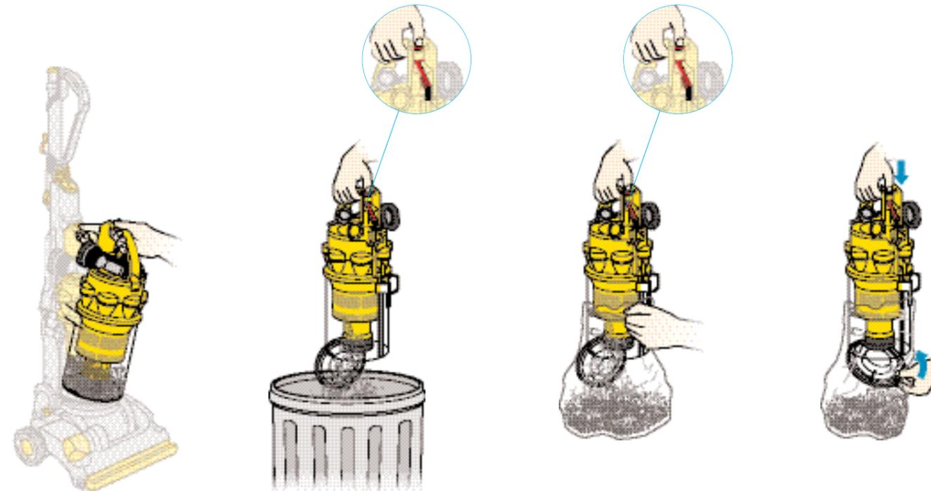
Empty the clear bin™ as soon as the **MAX** mark is reached. Press cyclone release button to release cyclone from machine.
