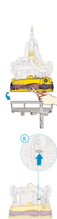
**B** Remove dirt or debris and check spindle is clean.
