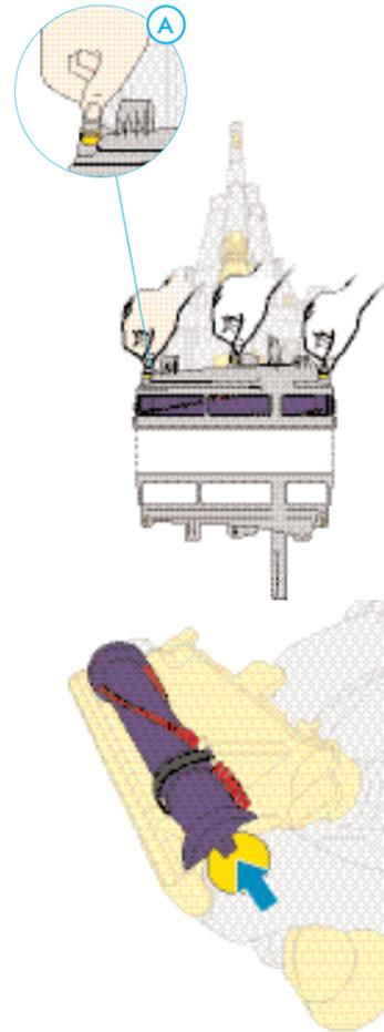
**A** Undo fasteners using a coin, slide back end caps and remove soleplate.
