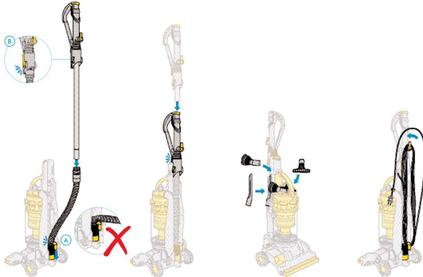
**A** Slide hose into guides at back of machine and click into place.
