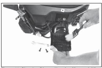
Figure 11. Cleaning Blower Housing Mounted Oil Cooler.
