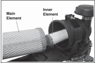
Figure 14. Removing Elements.
