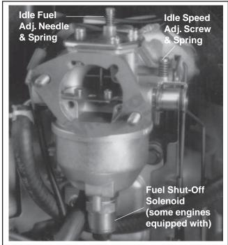
Figure 18. Carburetor CV17-25, CV675-740.
