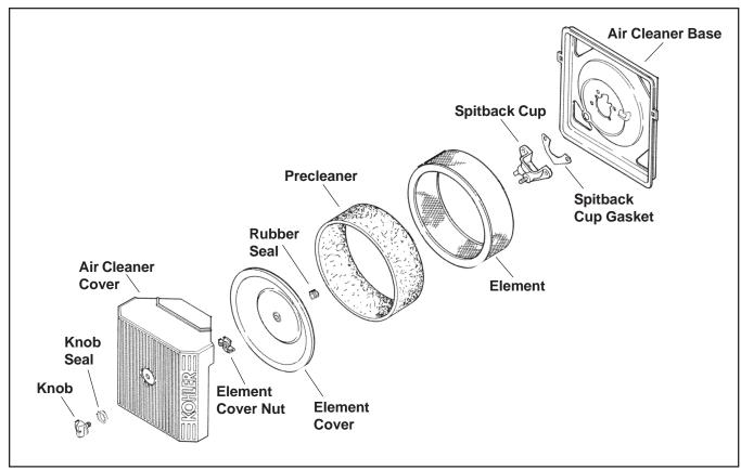
Figure 12. Air Cleaner System Components - Type A (Standard).
