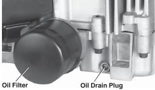
Figure 8. Oil Drain Plugs and Oil Filter.
