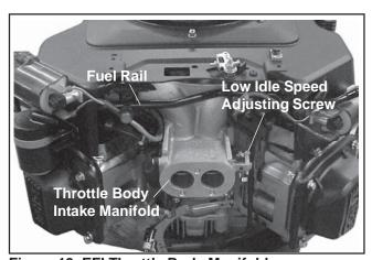
Figure 19. EFI Throttle Body Manifold.
