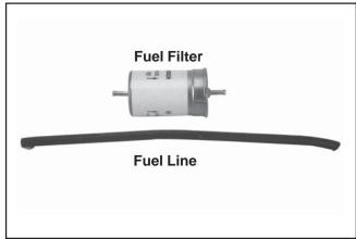
Figure 17. EFI Fuel Filter and Line.
