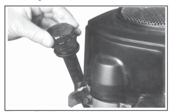
Figure 6. Checking Oil Level.
