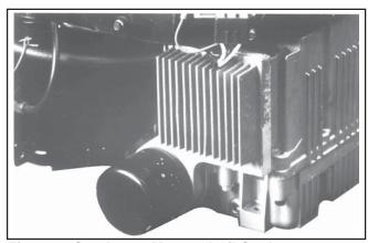
Figure 9. Crankcase Mounted Oil Cooler.
