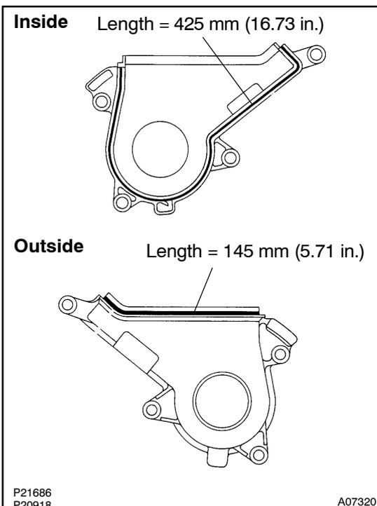
**12. INSTALL NO.1 TIMING BELT COVER AND STARTER WIRE BRACKET**
