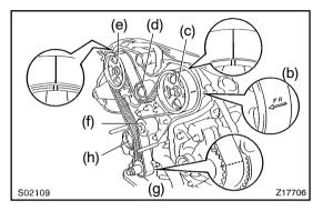
Using SST, turn the camshaft pulley, align the timing marks of the timing pulley and No.3 timing belt cover.
