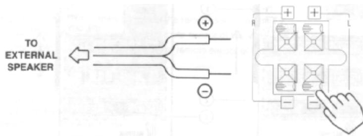
**CAUTION:** Do not connect Speakers simultaneously to the REAR SPEAKER terminal of the Projection TV and Amplifier. This could damage both the Projection TV and the Speakers. Your Hitachi TV was designed to use 8 $\Omega$  speakers only. Any other type may degrade the audio performance of your entertainment system.
