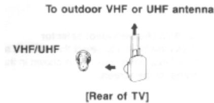
**When both VHF and UHF antennas are connected**
