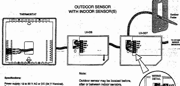
Probe operating temperature: -40 to 50°C. Sensor box operating temperature: 0 to 50°C, Sensor box maximum RH: 90% (non-condensing). Accuracy: +-2°C from -20 to 30°C (+-4°F from -4 to 86°F) after 30 minutes of continuous operation. Guaranteed measurement range: -30 to 47°C or -22 to 119°F. Maximum measurement range; -48 to 47°C or -55 to 116°F. Max. cable length between any 2 units; 300ft. (90m)
