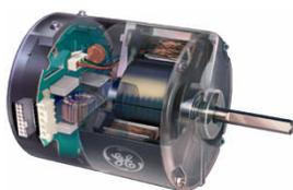
The GE ECM™ motor, currently used by most residential HVAC systems is a brushless DC, three-phase motor with a permanent magnet rotor. Motor phases are sequentially energized by the electronic control, powered from a single-phase supply. These motors are actually made of two components, a motor control (control module) and a motor, sometimes called a motor module.
