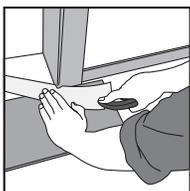
**[2]** Undercut doorjamb for a professional fit. Doorways less than 6' wide require T-Molding.
