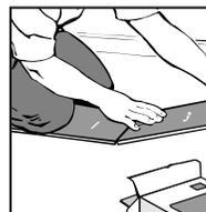
**[8]** Keep ends perfectly aligned while connecting the tongue and groove.
