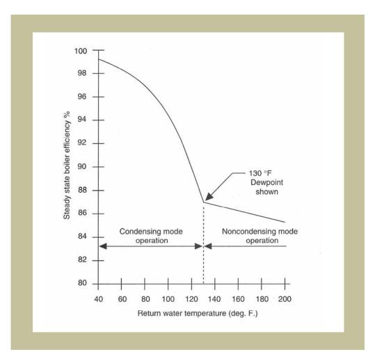
Figure 1. Boiler efficiency in both condensing and non-condensing modes. Source: Siegenthaler, Modern Hydronic Heating.
